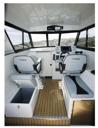
The fixed hardtop has a GRP internal liner for a real sense of class, side-opening windows for ventilation, and there was a toughened-glass windscreen with tinted side panes. Under the hardtop you'll find a handrail, radio box for the VHF and stereo, and storage compartments for personal effects. The boat's lighting plan included fluoros and trick LED cockpit lights, plus floodlights mounted on the hardtop for fishing.
